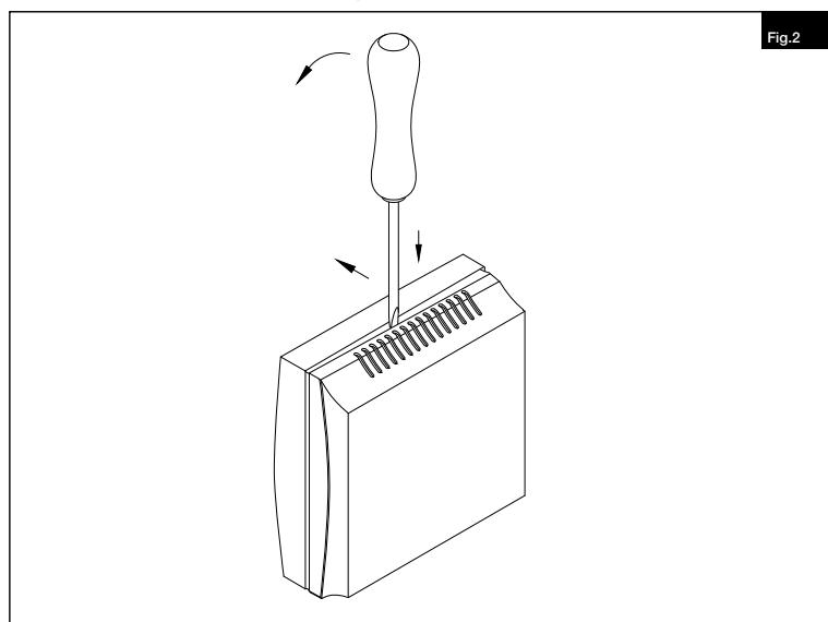
During subsequent assembly, hook in the snap-in hooks on one side of the housing base and snap in the housing.
