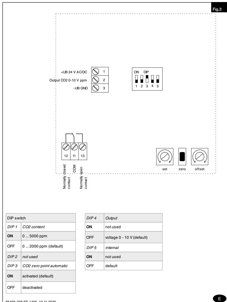
Maximum cable length between sensor and controls: 50 m.
